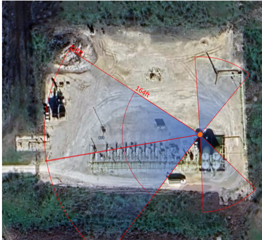
Figure 7: Example of overhead imagery of a facility, Kuva System placement, multiple fields-of-view of the camera and distance measurements.
