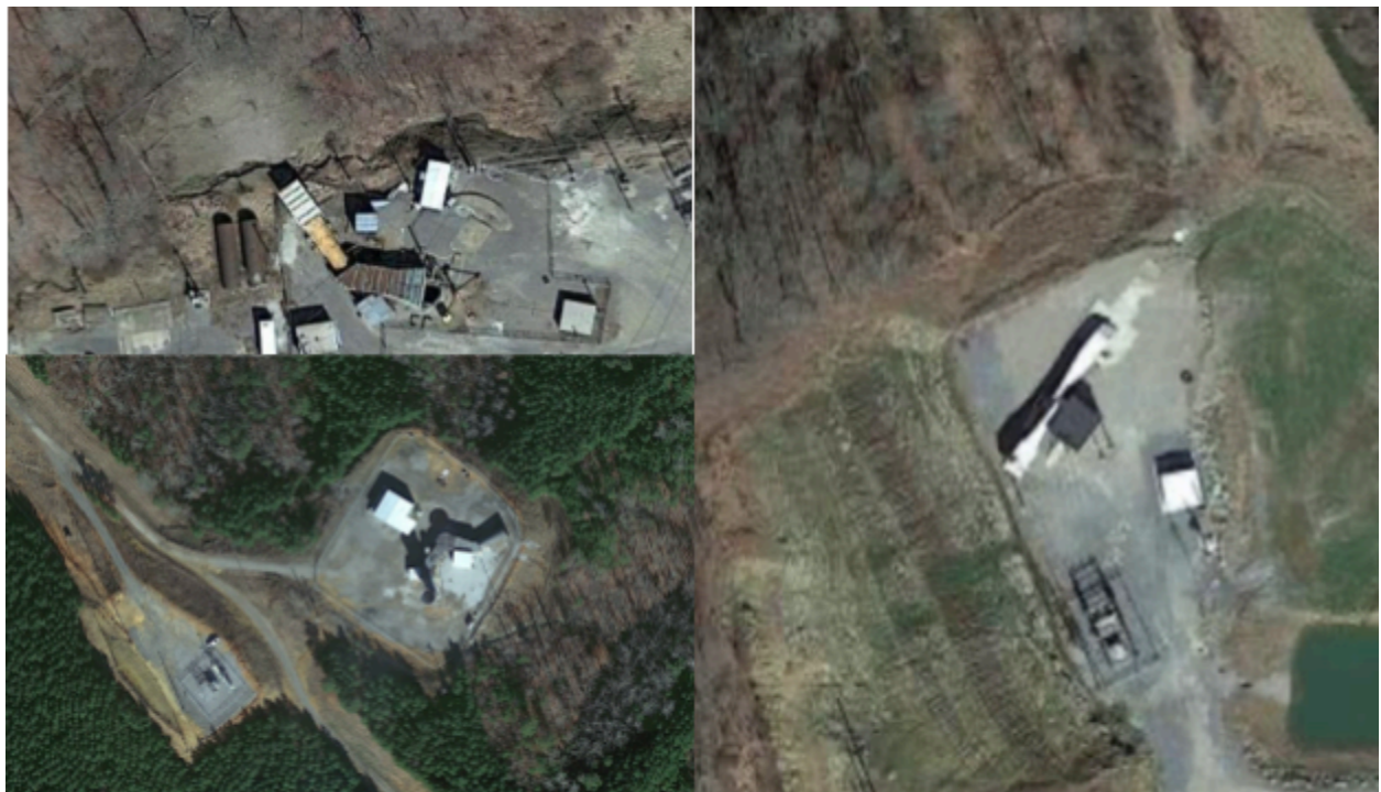
Figure 8: Basemap image in the left panel and gaussian plume in the right panel coming from a coal vent. Underground mines often have very strong and discreet plumes, however the vent can sometimes be hard to spot in base map images
