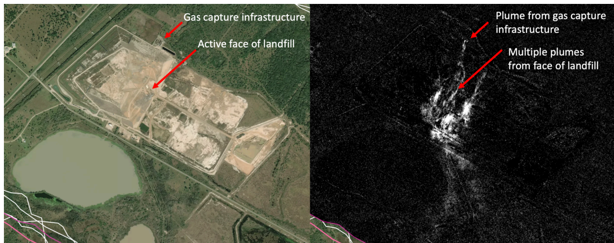
Figure 15: Example of multiple plumes at a single landfill. One plume originates from the gas capture infrastructure at the landfill, and multiple plumes originate from the active face of the landfill where trash is being deposited.
