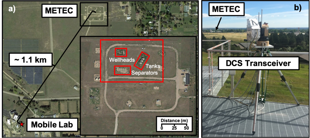
Figure 1: Overview of the METEC test site and the DCS sampling location (panel a) and a photo of the DCS transceiver (panel b). Panel a) the red star indicates the position of the DCS at the foothills campus of Colorado State University, which is ~1.1 km away from the METEC site. The inset includes a closer view of METEC, with the red squares highlighting the different potential source regions: 1) a battery of 5 wellheads; 2) a battery of 4 separators; and 3) a battery of 3 tanks. Panel b) contains a picture of the DCS transceiver with the METEC site noted in the background. The larger red square in the inset corresponds with the region shown in figure S1. panel a.
