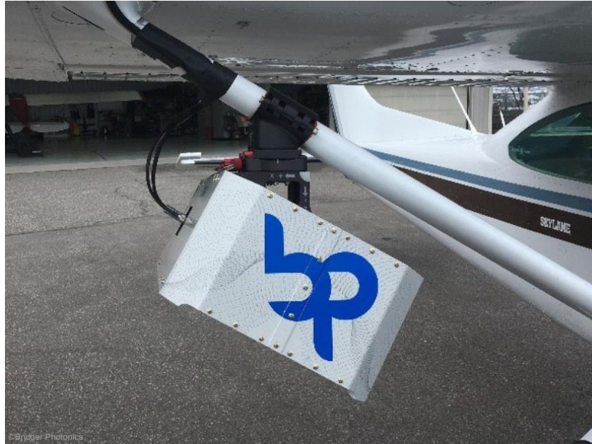
Figure 2. A GML 2.0 instrument mounted to the strut of a fixed-wing aircraft.
